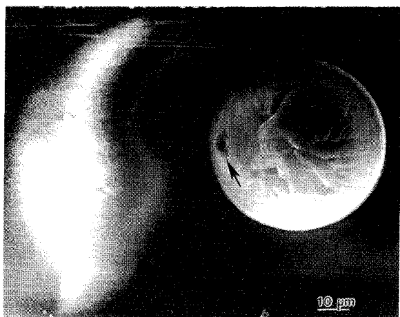
Fig. 9 SEM micrograph of a 70- \mu m aluminum particle quenched approximately 5.5 ms after ignition.
